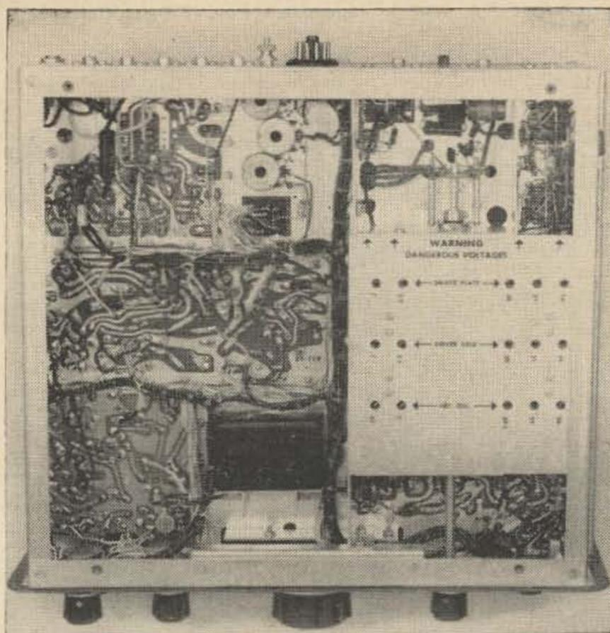
cuit boards, each with a switch wafer and associated components, that is used for the bandswitch.
