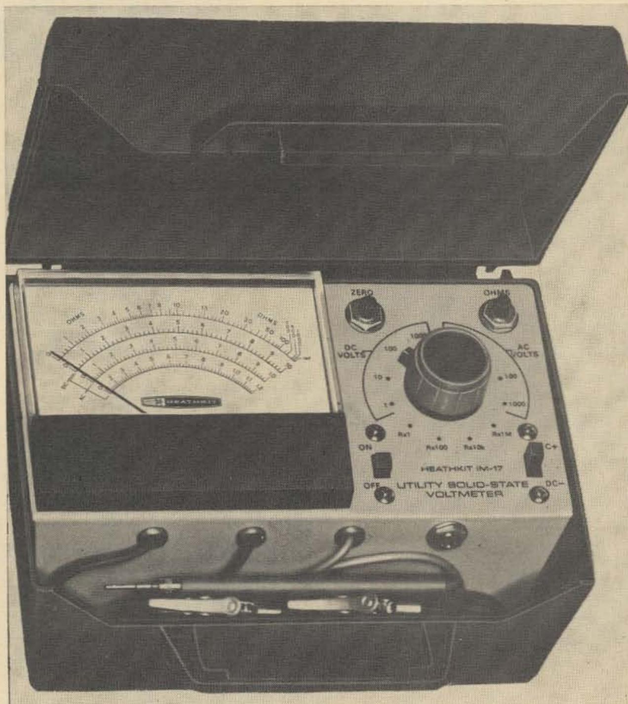
Still tied to the 110-volt line with a VTVM? After several hours of hunting for my test leads, pulling out an extension cord, warming up of the VTVM, I decided to invest in a good solid state voltmeter. At a price lower than most VOM's the Heath-IM-17 fills the bill for a high impedance voltmeter.
