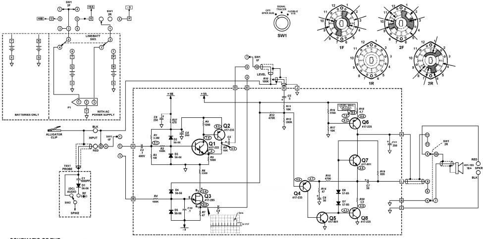
SCHEMATIC OF THE HEATHKIT MODEL IT-5283 SIGNAL TRACER
