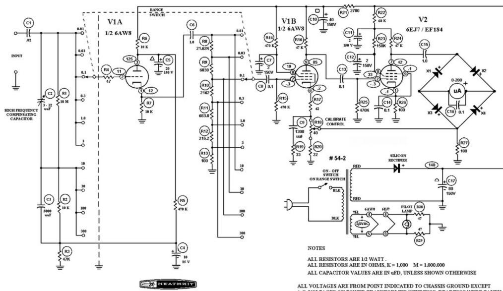
AC VACUUM TUBE VOLTMETER
