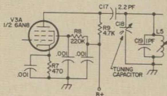
Unmodified Sixer receiver, rf stage.
