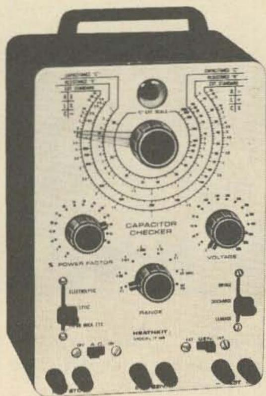
A careful scanning of most of the electronics magazines from the early '50s to the present has brought to light some interesting capacitor checker circuits, but none of the construction articles on these instruments boasted a range from picofarads to hundreds of microfarads.<sup>1,2</sup> This is the range encountered by even a casual builder.
