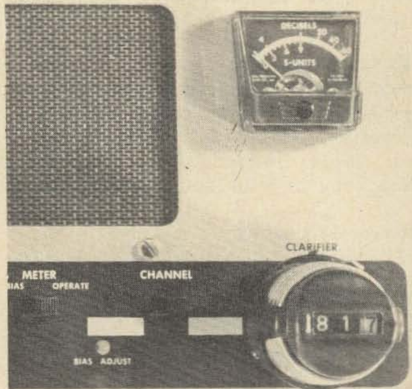
This inexpensive digital dial readout is nice.
