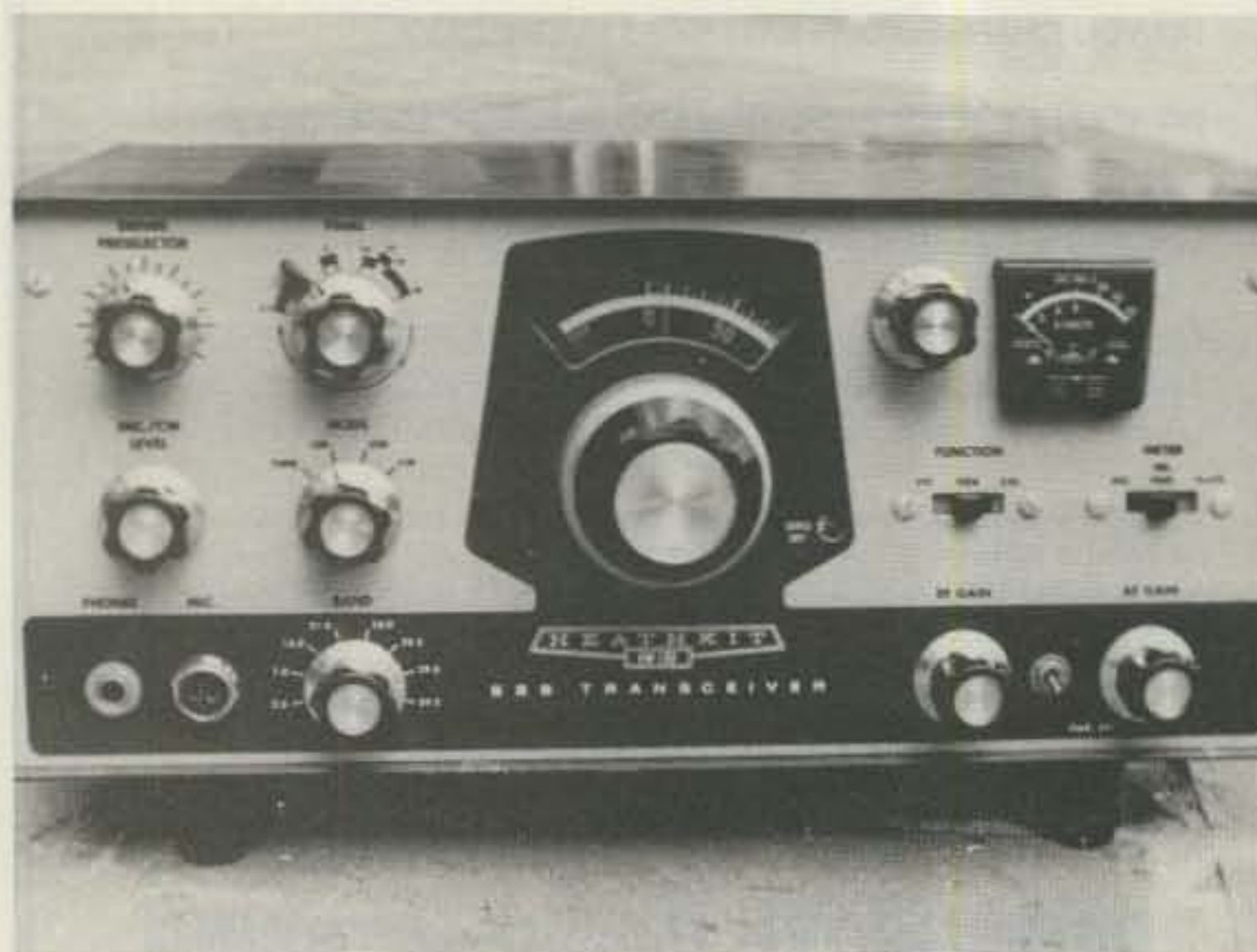
Photo A. The HW-100 with added Swan dial and audio-response control on the upper right. The small toggle switch on the lower right controls an external antenna relay.
