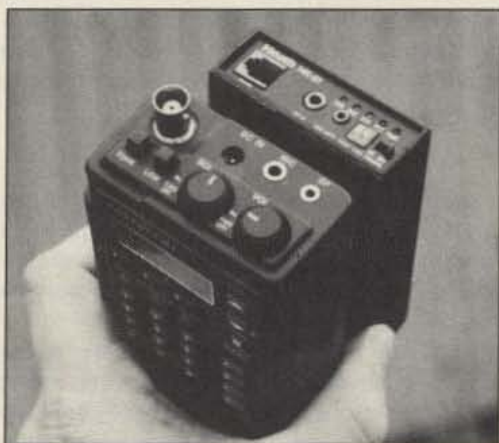
Photo C. The HT and TNC fastened together. Note the phone jack.
